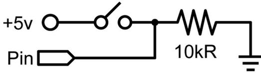
This is the simplest form of input with only two possible states: on or off. This example reads a simple switch or pushbutton connected to pin2. When the switch is closed the input pin will read HIGH and turn on an LED.
