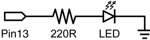
This is the basic 'hello world' program used to simply turn something on or off. In this example, an LED is connected to pin13, and is blinked every second. The resistor may be omitted on this pin since the Arduino has one built in.
