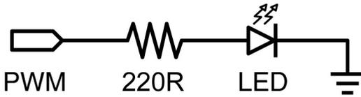
Pulsewidth Modulation (PWM) is a way to fake an analog output by pulsing the output. This could be used to dim and brighten an LED or later to control a servo motor. The following example slowly brightens and dims an LED using for loops.
