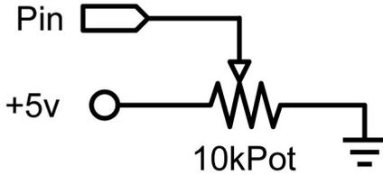
Using a potentiometer and one of the Arduino's analog-to-digital conversion (ADC) pins it is possible to read analog values from 0-1024. The following example uses a potentiometer to control an LED's rate of blinking.
