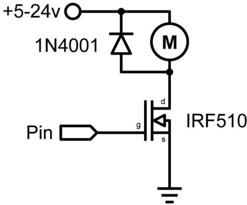
Sometimes it is necessary to control more than 40ma from the Arduino. In this case a MOSFET or transistor could be used to switch higher current loads. The following example quickly turns on and off the MOSFET 5 times every second.
